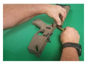
Caution: Buffer is under tension from action spring.
