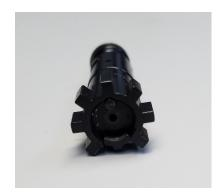
2. Take a fired or dummy case and place it under the lip of the extractor. With a rocking motion, press the case down against the ejector. Since the ejector is spring loaded some resistance will be felt. Press on the case until it stops against the bolt face. Ease off with your thumb slightly and press down again. Repeat several times. Replace the CLP frequently. Once the spring action of the ejector is smooth and strong dry off any excess lubricant
