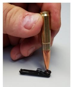
CHECK THE BOLT: Look for cracks or fractures, especially in the cam pin hole area. Inspect bolt face. Bolts with any pitting extending into the firing pin hole should be replaced.
