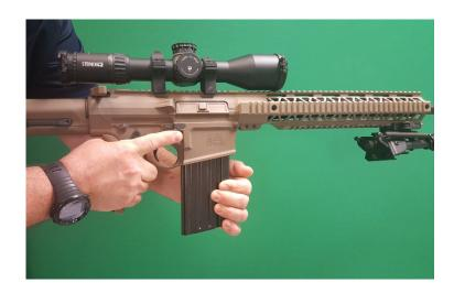
2. Slap upwards on magazine bottom to make sure it is seated correctly.
