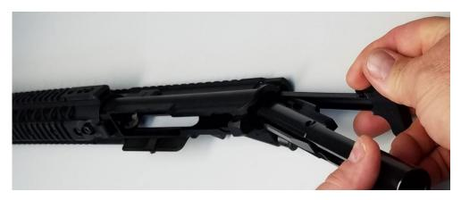
9. Lower complete bolt carrier assembly into upper receiver. Gas key will fit into groove in the charging handle. REMEMBER bolt must be pulled to "out" position in the carrier so cam pin will fit into the channel in the upper receiver.
