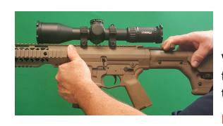
With a magazine in the rifle, pull the charging handle fully to rear then release the charging handle allowing the bolt to spring forward -chambering the first round.
