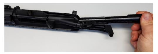
10. Then slide the bolt carrier assembly and charging handle all the way into the upper receiver until charging handle latch locks onto the receiver.
