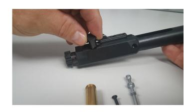
11. Remove bolt assembly from bolt carrier by pulling straight out.
