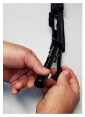
**NOTE**: If ejection port cover is closed, you will feel some resistance as you push carrier and handle in until you pop the cover open. If cover is already open, handle and carrier should slide in easily.
