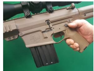
3. Place Selector Lever in FIRE position. Pull the Trigger. THE HAMMER SHOULD FALL
