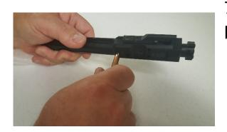
7. Remove firing pin retaining pin. A bullet tip can help push it out.
