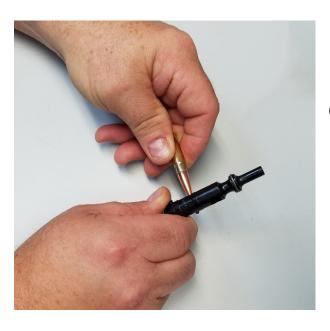
12. Remove extractor pin by pushing out with a punch or the tip of a bullet.
