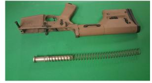
receiver extension and latch mechanism to ensure proper telescoping action. A2 solid buttstocks may require cleaning or lubrication of storage compartment door latch and hinge and interior of storage compartment.
