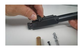
10. Remove cam pin by rotating ¼ turn and lifting out.
