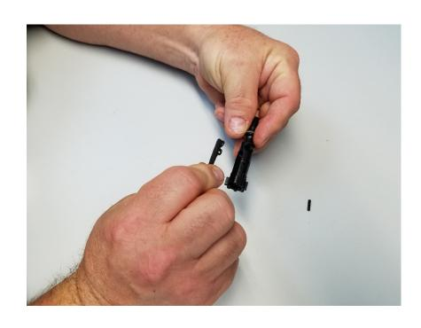
Note: Check spring function by pressing rear of extractor
